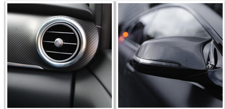
Examples of small CFRTP parts with complex structure
